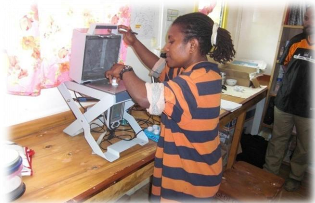
Niton XRF Analyser in Operation at Yandera
